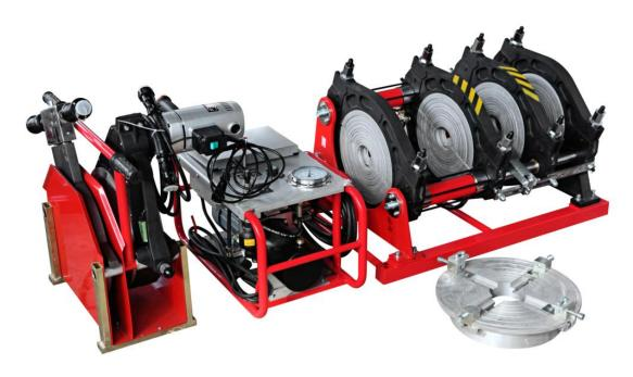
◆ Welding ranges: plastic pipes: 90--315mm
